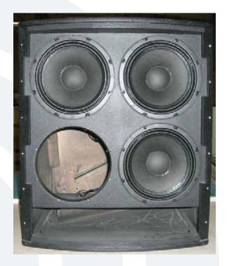
The picture above shows what the S410s looks like with the grill and bottom left woofer removed. Place the new woofer (part #0011737) where the old one was. Follow the same steps as above, but backwards 4 to 1. Power up the S410s and the new woofer should now be pumping out glorious lows. Awesome, you just replaced a 10" woofer!
